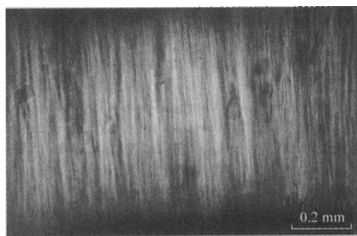
Fig. 7. Photomicrograph of the chain structures formed by aminopropyl group-modified silica particles in silicone oil in a dc electric field.
